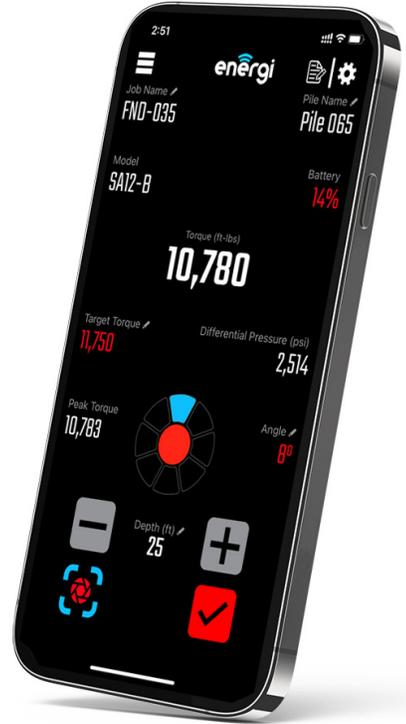
All recorded data is formatted into a user-friendly preformatted PDF reports. All recorded jobs include a Summary Report which provides an overview of the entire job and Individual Pile Reports that provide in-depth installation data on each helical pile.
